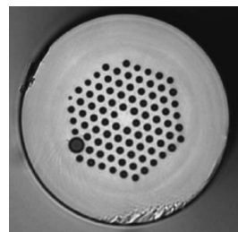
Fig. 27 PCF cross-section of endlessly single mode fiber with inherent asymmetry.
