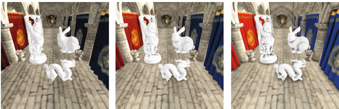
Fig. 6 With 24 spp. Left: Illuminated by Phong shading using uniform ambient light (51 FPS). Middle: Illuminated by Phong shading using the Mittring [2] SSAO method (47 FPS). Right: Our SSAO MIS technique with Phong shading (47 FPS)
