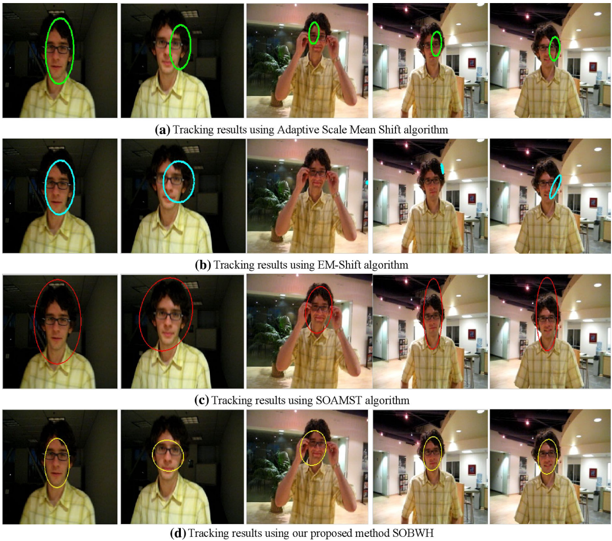
Fig. 5 Tracking results from “David” sequence for frames 2, 9, 296, 439 and 471 are displayed. a Tracking results using Adaptive Scale Mean Shift algorithm, b tracking results using
