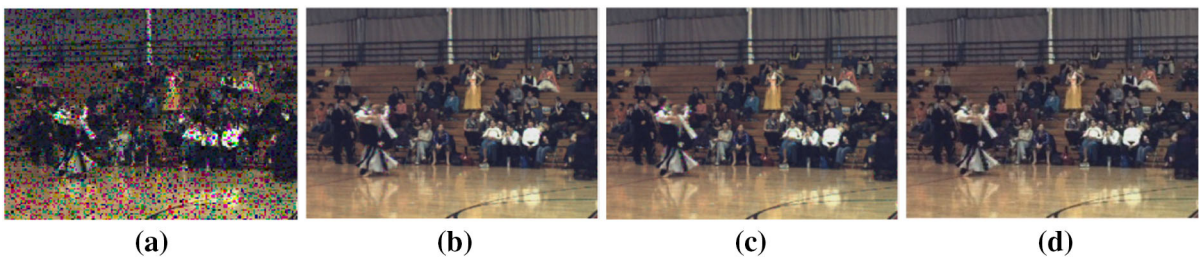
Fig. 6 Subjective simulation results for the selected 209th intra I-frame within I-view S_0 of the “Ballroom” sequence at channel SNR = -5 dB: a Erroneous I_{209} with SNR = -5 dB,
