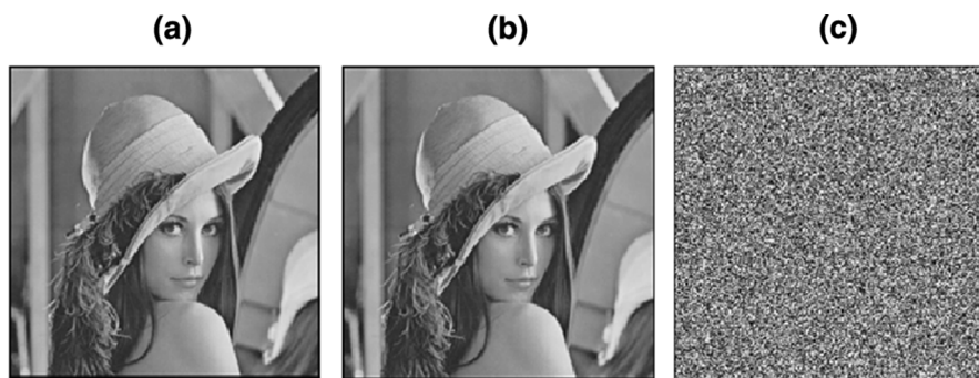
Fig. 6 Key sensitivity test for the decryption process for the Lena image. a original image b decryption with the correct key c decryption with the slight changed key
