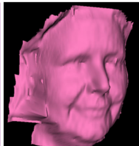
3D shaded, 3D RMSE=3.95 Scale=3 with DCT 8x8 [Compressed size 6.74 Kbytes]
