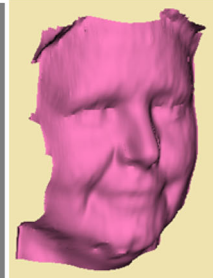
3D shaded, 3D RMSE=3.39 Scale=5 with DCT 8x8 [Compressed size 6.37 Kbytes]
