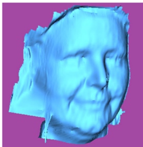
3D shaded, 3D RMSE=2.46 Scale=2 with DCT 8x8 [Compressed size 9.7 Kbytes]
