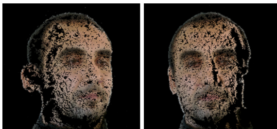
Fig. 14 Two views of the results of the 3D reconstruction by using a binocular stereovision system
