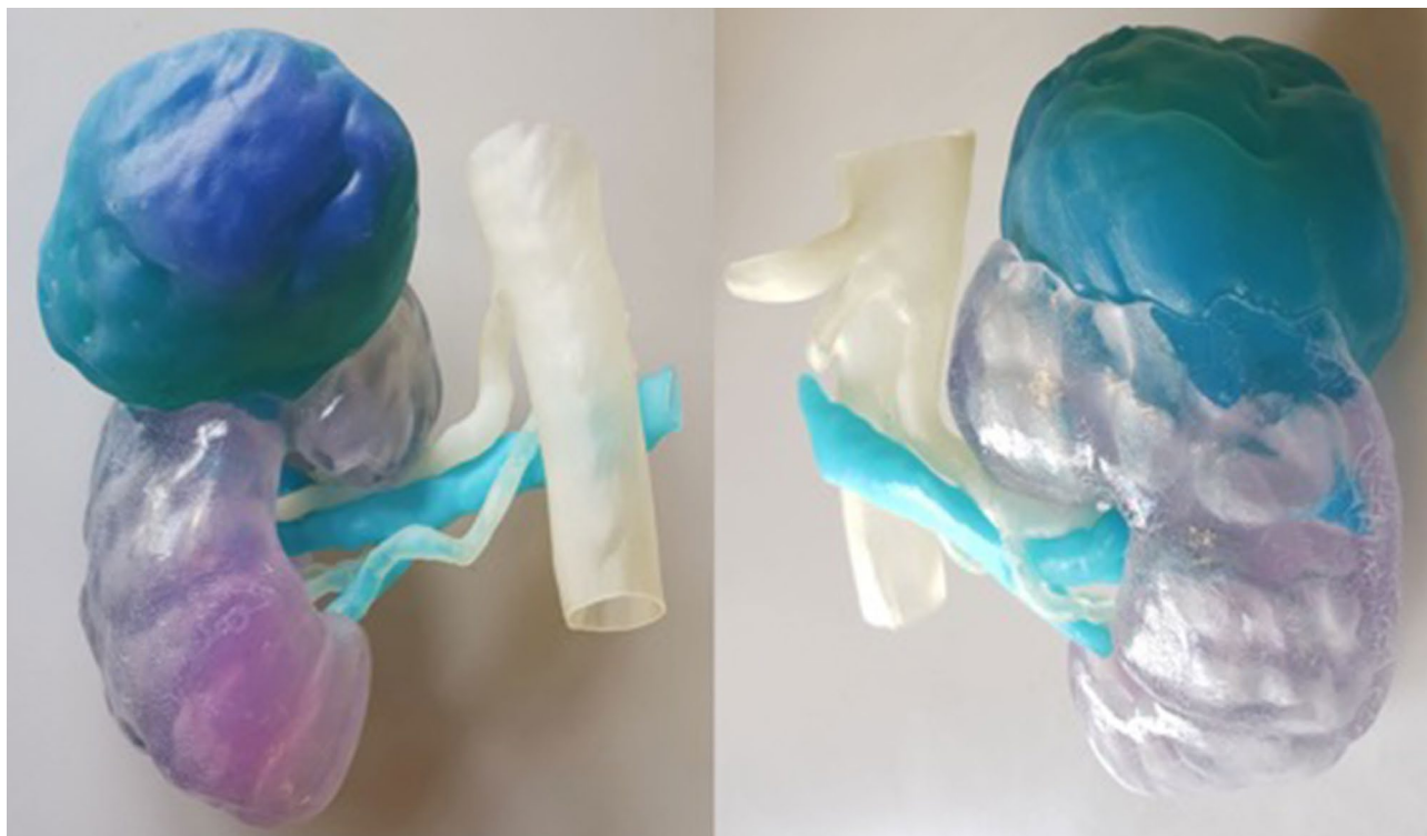
Fig. 2 3D printed model, made of photopolymer resin using a Material Jetting printer (Objet 260 Connex 3—Stratasys), showing a left adrenal gland tumor and its relationship with the corresponding kid-
