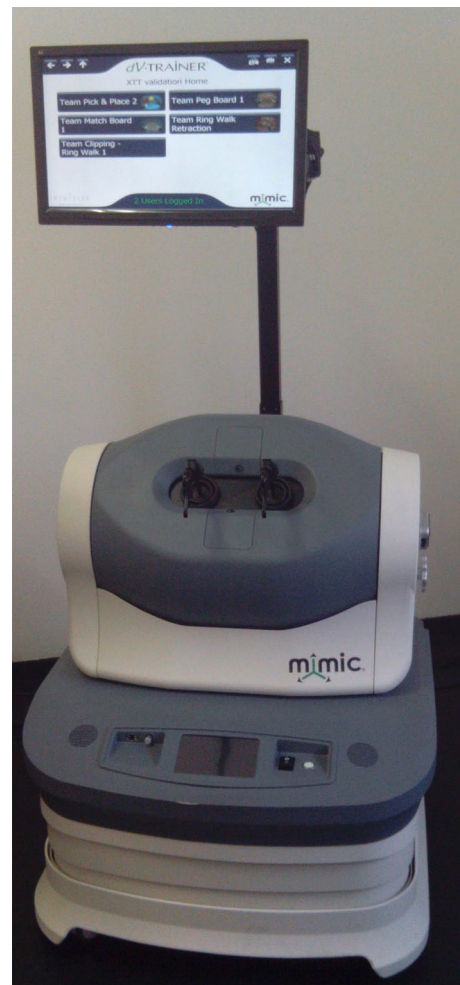
Fig. 1 Xperience™ Team Trainer platform Xperience™. Team Trainer (Mimic Technologies, Inc., Seattle, WA) is a virtual reality simulator available as an optional hardware component for the dv-Trainer® and simulates the patient-side working environment. It consists of a platform with two movable laparoscopic tool ports with force feedback capability and width adjustment, an integrated video monitor, and it is equipped for ergonomic height adjustment and rotation and tilt adjustment supporting common port positions used in robotic procedures. The surgical simulation software used is M-Sim™ 3.0 (Mimic Technologies, Inc., Seattle, WA)
