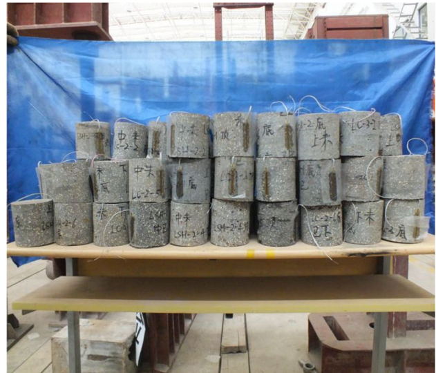
Fig. 2 Standard cylinder specimens
