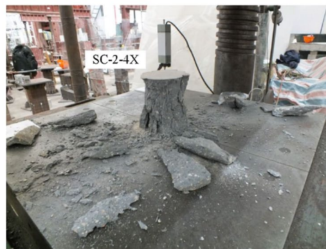
(c) Specimen on the compression machine after test
