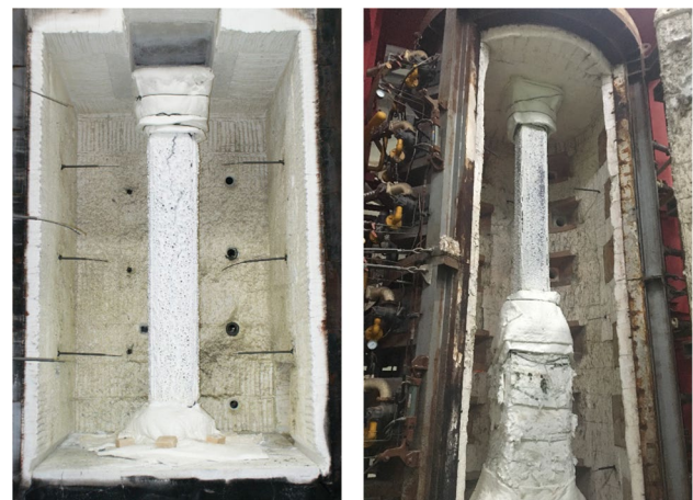
(a) Non-loading test (b) Loading test
