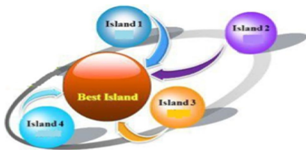
Fig. 1 Migration of the selected designs to the best island in multi meta-heuristic-based search method (MHSM)
