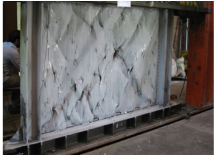
Fig. 4 Comparison of tested by Emami et al. (2013) and finite element model: a Hysteresis curves and b Failure modes
