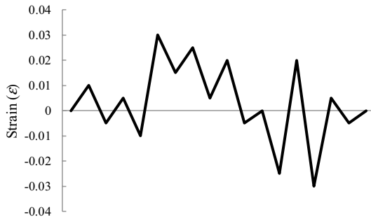
Fig. 4 Programmed loading history (Specimen SA440_P)
