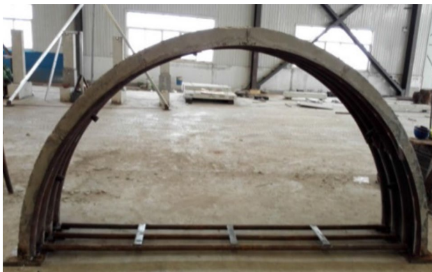
Fig. 6 CSP-concrete arch model
