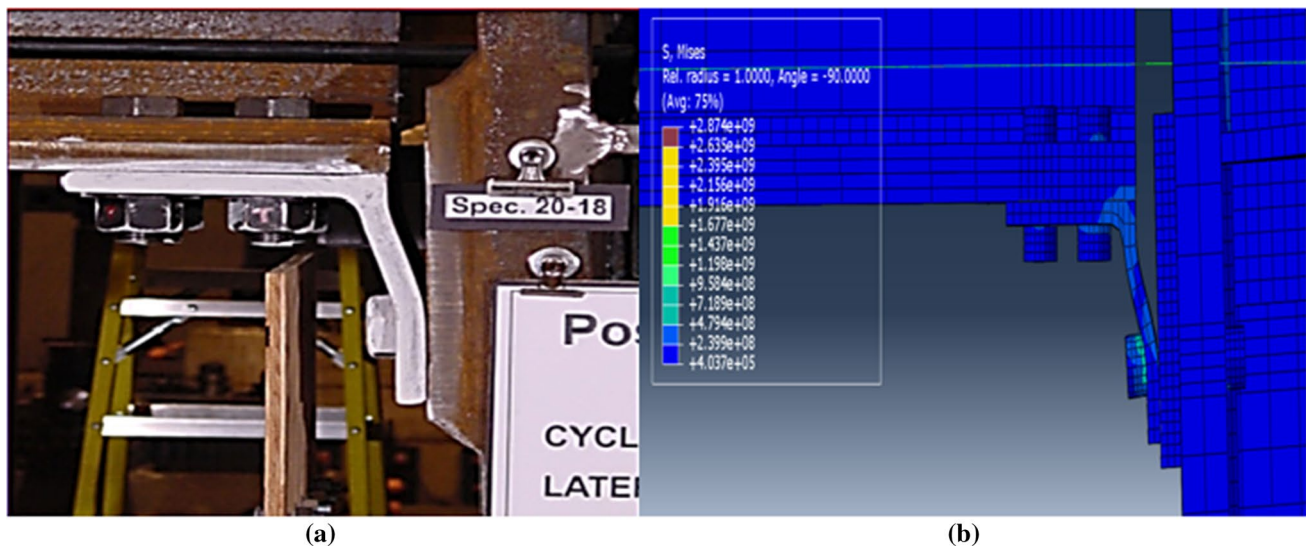
Fig. 8 PT connection in a experimental analyses by Garlock et al. (2005) (36s-20-P). b Finite element analyses at 4% drift ratio
