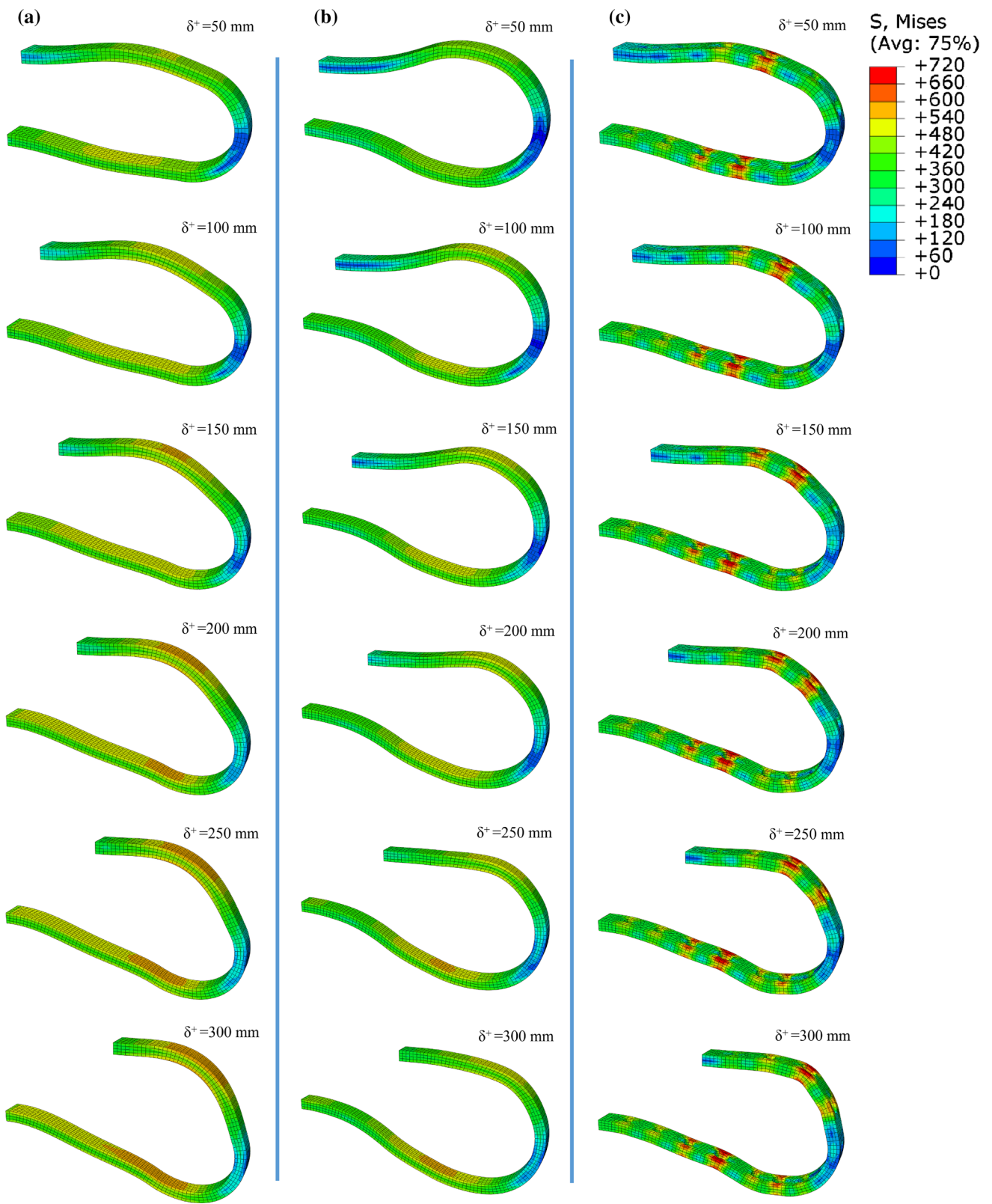
Fig. 10 Stress distributions and deformed shapes under 0^\circ loading a UD-S, b UD-N1 and c UD-P1
