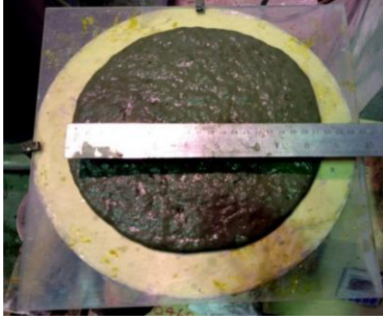
Figure 3. Flow table test of ULCC.
