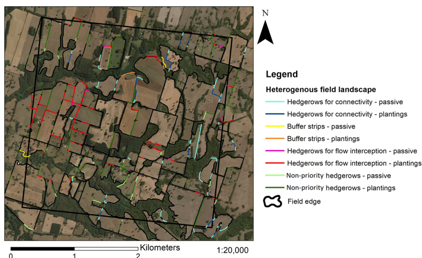
Fig. 4 Proposed restoration scheme of the buffer strip and hedgerow network in the 3 \times 3 -km agricultural landscape that is representative of fields of heterogeneous size
