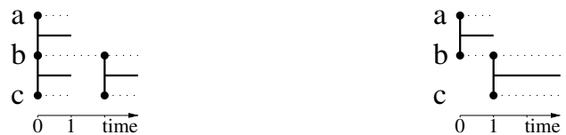
Fig. 2 Two stream graphs with n = 2 nodes, m = 1 link, but with different densities: Left: \delta = 0.75 . Right: \delta = 1
