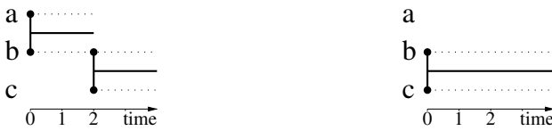
Fig. 6 These two stream graphs have density 1 (all possible links exist), 2 nodes, and 1 link. However, the leftmost one has average node degree d(V) = \frac{|T_a|}{|W|}d(a) + \frac{|T_b|}{|W|}d(b) + \frac{|T_c|}{|W|}d(c) = \frac{2}{8}0.5 + \frac{4}{8}1 + \frac{2}{8}0.5 = 0.75 and the rightmost one has average node degree 1
