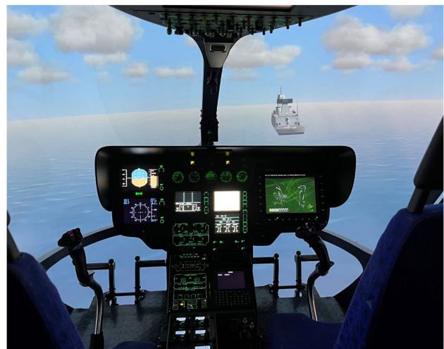
Fig. 2 DLR's simulator-Cockpit point of view during maritime simulation
