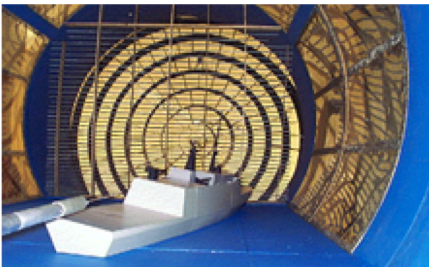
Fig. 5 Ship air-wake measurements at IMFL wind tunnel facilities
