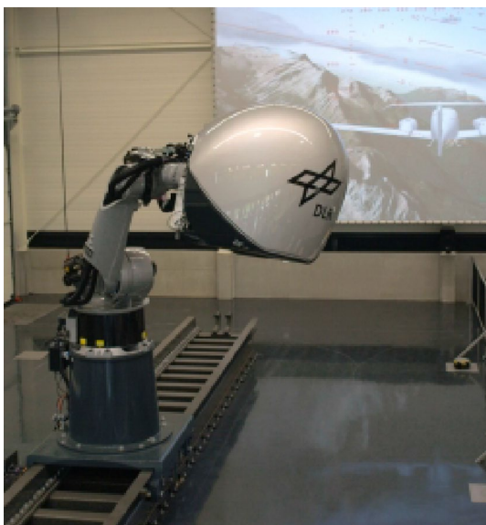
Fig. 12 Robotic motion simulator at the DLR Institute of system dynamics and control [3]
