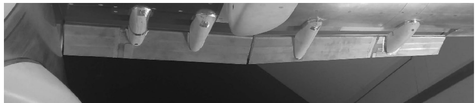
Fig. 17 Lined flap mounted on the left wing in LA configuration
