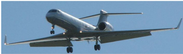
(b) Flaps deflected 39^\circ with main and nose gears deployed; left image 2006 flight test, right image simulated CAD model
