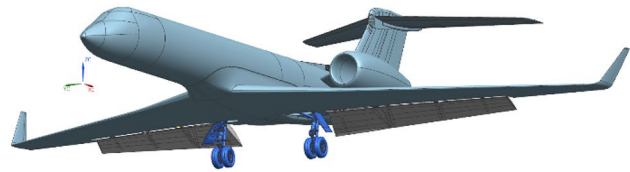
(a) Flaps deflected 39^\circ with main gear deployed; left image 2006 flight test, right image simulated CAD model
