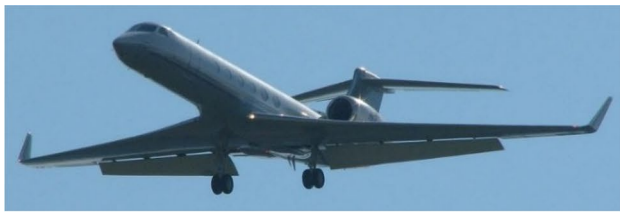
(a) Flaps deflected 39^\circ with main gear deployed; left image 2006 flight test, right image simulated CAD model
