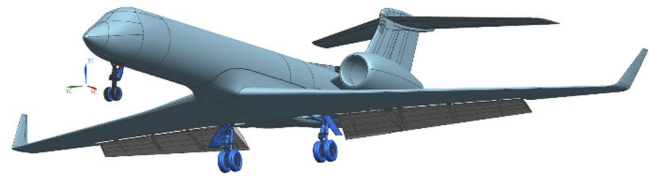
(b) Flaps deflected 39^\circ with main and nose gears deployed; left image 2006 flight test, right image simulated CAD model
