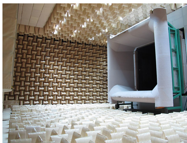
Fig. 7 Open-jet test section with anechoic plenum of DNW-NWB
