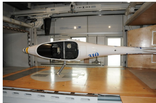
Fig. 2 Sting-mounted aircraft fuselage in the test section of the wind tunnel A of the Technical University of Munich [26]
