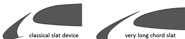
Fig. 9 The very long chord slat (VLCS)—a concept to reduce slat trailing edge noise at comparable aerodynamic performance
