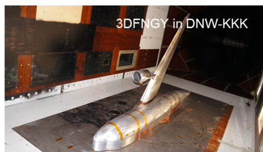
Fig. 11 The very long chord slat (VLCS) applied to 3D half model installed in the DNW-KKK cryogenic wind tunnel for testing at higher Reynolds number (image from [24])
