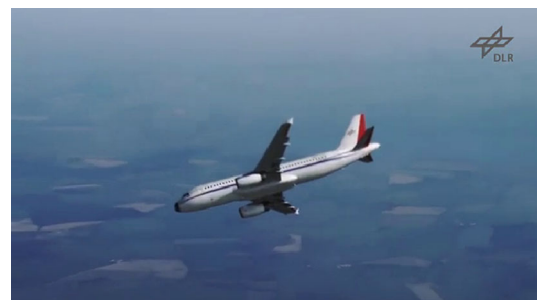
Fig. 1 DLR research aircraft ATRA diving just past stall (image extracted from [13])
