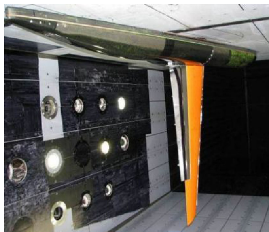
Fig. 4 DLR-F11 high-lift model equipped with laminar wing high-lift system (DS21) in the test section of the ETW (image from [16])
