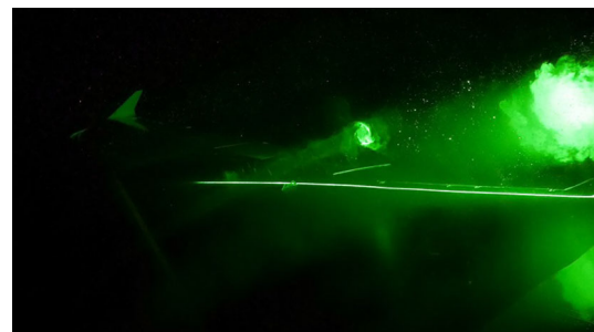
Fig. 2 Application of in-flight PIV to trace vortices close to stall conditions (image: http://www.dlr.de )
