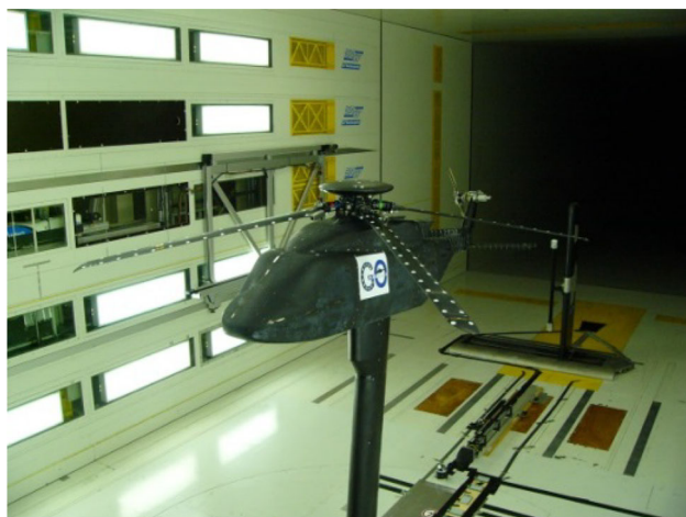
Fig. 30 Wind tunnel set-up in GOAHEAD
