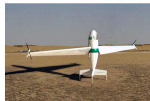
Fig. 3 Tazenflugel with tilted wings [8]
