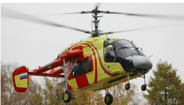
Fig. 23 Kamov Ka-226 in HEMS configuration. Source: Russian Helicopters, http://www.russianhelicopters.aero/en
