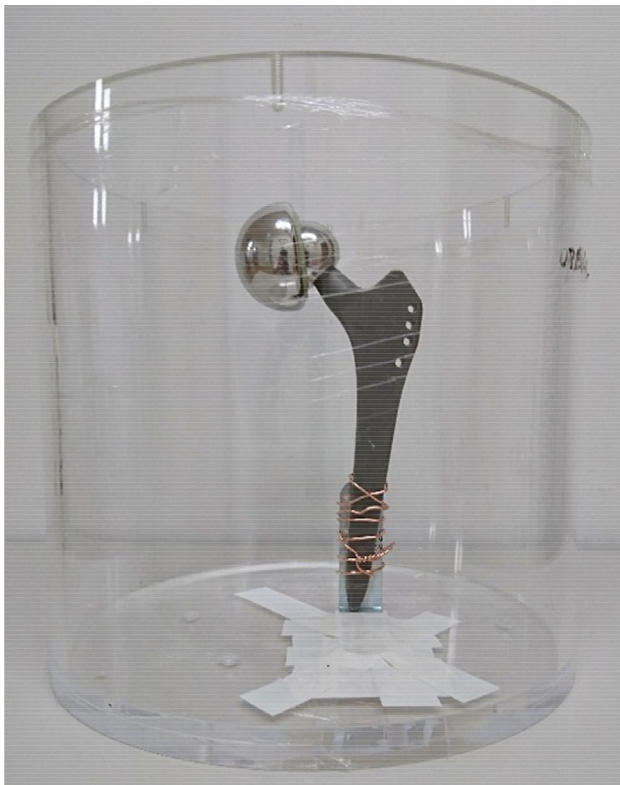
Fig. 1 The phantom with artificial hip joint in the center
