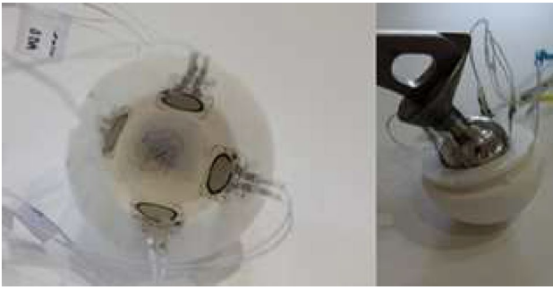
Fig. 6 Positions of force sensors in the acetabular liner
