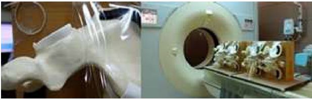
Fig. 11 Four pelvic bone models with randomized attaching acetabular cup in different angles
