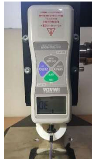
Fig. 4 Force gauge and the direction of force while calibrating
