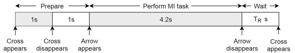
Fig. 1 Top -The timeline of a single trial of MI experiment. Bottom -The cue displayed to instruct the subject to imagine right-hand clenching MI
