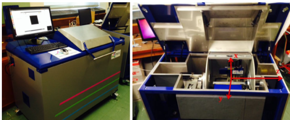
Fig. 1 Photograph of the MARS scanner exterior and the interior with the covers open. The spatial axes of the gantry are indicated
