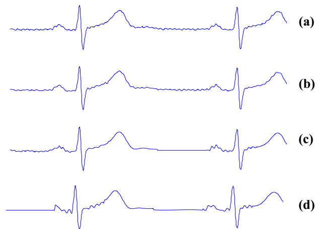
Fig. 3 Original signal and reconstructed signal segment of record no. 117 at different PRD for quantization resolution of 8 bit for 30 min duration. a Original data. b CR = 10.92, PRD = 0.30, UPRD = 0.2 and TH = 5.14. c CR = 16.64, PRD = 0.45, UPRD = 0.4 and TH = 15.21. d CR = 23.57, PRD = 1.01, UPRD = 1 and TH = 46.66
