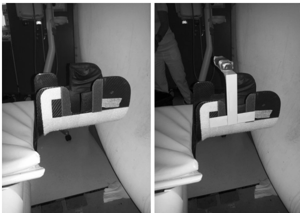
Fig. 1 Developed height adjustable system for shielding set-up
