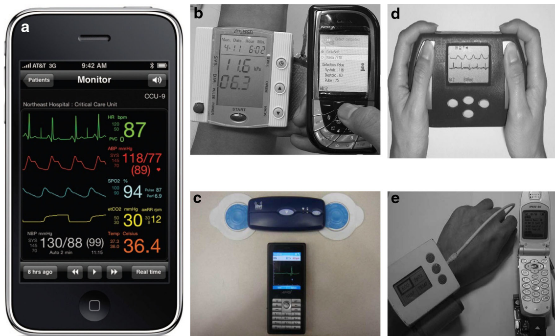
Fig. 1 a Image courtesy of AirPort Technologies [45], b a mobile healthcare system with alert mechanism developed by Ren-Guey et al. [47], c HeartToGo—a cardiovascular disease detection system developed by Oresko et al. [3], d a remote patient monitoring system
