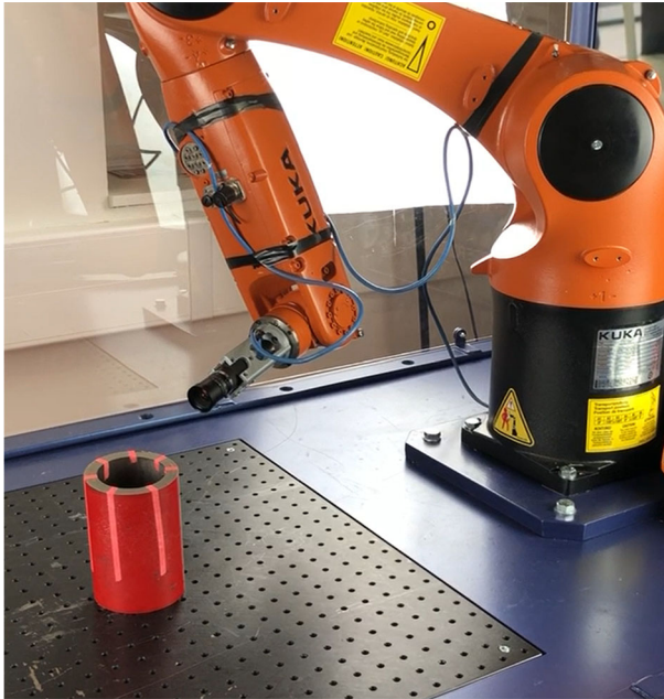
Fig. 3 Industrial machine vision camera attached to the end effector of KUKA AGILUS
