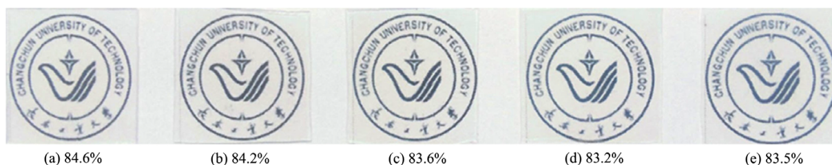
Figure 9. Transparency of (a) pure poly(St-BA) film and (b) polymer/SiO 2 nanocomposite films with the different SiO 2 contents (b) Si-0, (c) Si-1, (d) Si-2, (e) Si-3.
