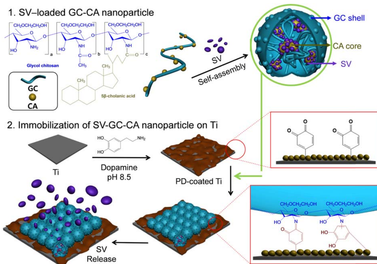
Figure 1. Schematic illustration of preparation of SV-loaded GC-CA nanoparticles, nanoparticle immobilization onto PD-coated Ti substrates, and the sustained release of SV.
