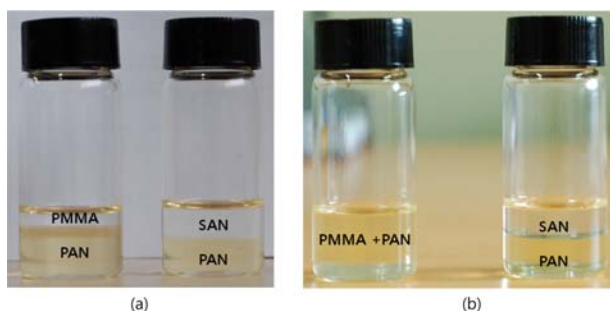
Figure 5. Mixing behavior of the PMMA and SAN solutions with the PAN solution. (a) as-poured and (b) after one day.
