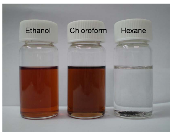
Figure 5. Dispersion behavior of \text{Fe}_3\text{O}_4\text{-OAm-Aphen} nanoparticles in various solvents.
