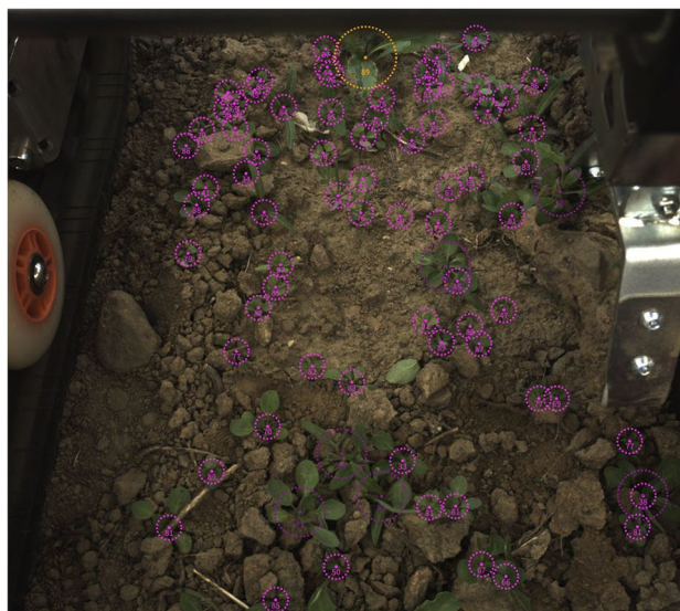
Fig. 6 Labeled image from Learning Loop with detections. Classes were sugar beets (orange), weed (pink) and big weed (purple)
