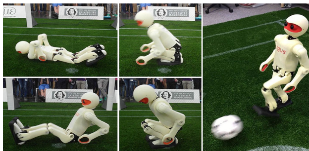
Fig. 4 Dynamic get-up motions of the igus ® Humanoid Open Platform, from the prone (top row) and supine (bottom row) lying positions, and a still image of the dynamic kick motion
