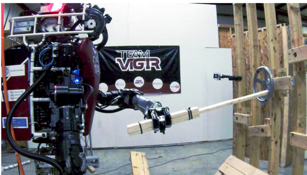
Fig. 4 The supervisor is able to command the robot to execute the valve turn affordance, however because of debris blocking the way, the supervisor is utilizing a stick to achieve the task [14]
