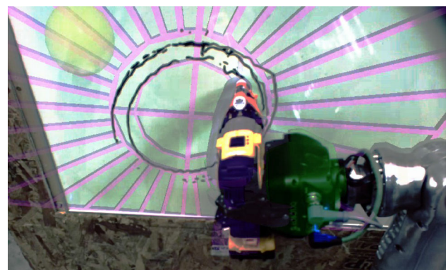
Fig. 7 Team ViGIR's Atlas robot's first person view of the Draw Circle in the Wall task. An ovoid shape pattern can be appreciated which is generated due to joint controller inaccuracies generated by the drill mass, which is around 1.3 kg
