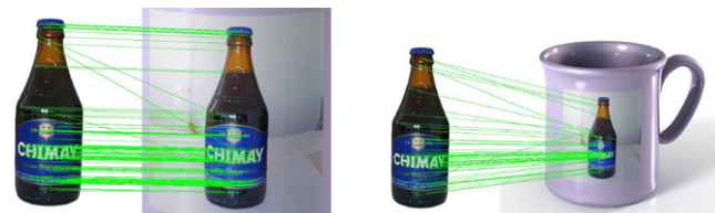
Fig. 2 An example of a good model match using features extracted from 2D images (left), where an object template is successfully identified in an image. However, zooming out from the image, we observe that the template is in fact another picture stitched to a completely different 3D object (in this case a mug). The semantics of the objects in this case are thus completely wrong
