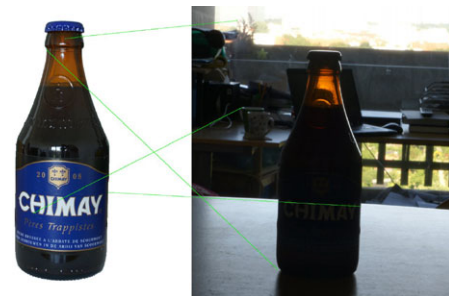
Fig. 1 Model matching failure in underexposed 2D images. None of the features extracted from the model (left) can be successfully matched onto the object of interest (right)
