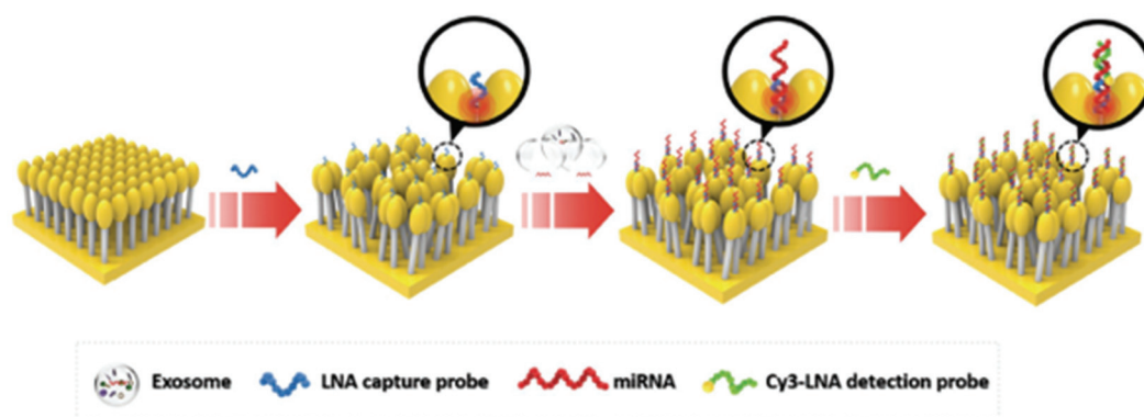
Figure 5. Schematic diagram of exosomal miRNA detection using head-flocked nanopillar SERS substrates. LNA capture probes were immobilized on the head-flocked nanopillar SERS substrate followed by capturing target miRNAs. Subsequently, Cy3-LNA detection probes were also bound to the target miRNAs. Hybridization of perfectly matched LNA capture probes-target miRNAs-LNA detection probes generated strong Cy3 Raman signal by hot spot inside of head-flocked nanopillar structures 65 . Images reproduced with permission from [65].
