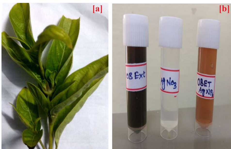
Fig. 1 Colour changes of biosynthesized OBETAgNPs from Ocimum basilicum L. The first tube in extreme left indicates OBET Extract (before adding \text{AgNO}_3 ); middle is after adding \text{AgNO}_3 and the later is stabilized AgNPs after 12 h of reaction time
