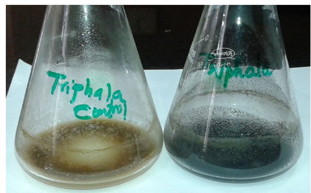
Fig. 1 A qualitative method to detect the presence of tannins in the substrate Triphala . Development of brownish green or blue–black coloration indicates the presence of tannins
