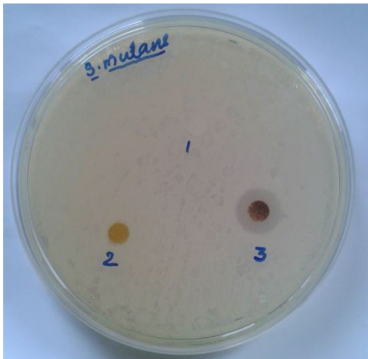
Fig. 7 Disc diffusion assay against Streptococcus mutans of (1) neat PMMA membrane (2) PMMA with CAgNPs (3) PMMA with MAgNPs
